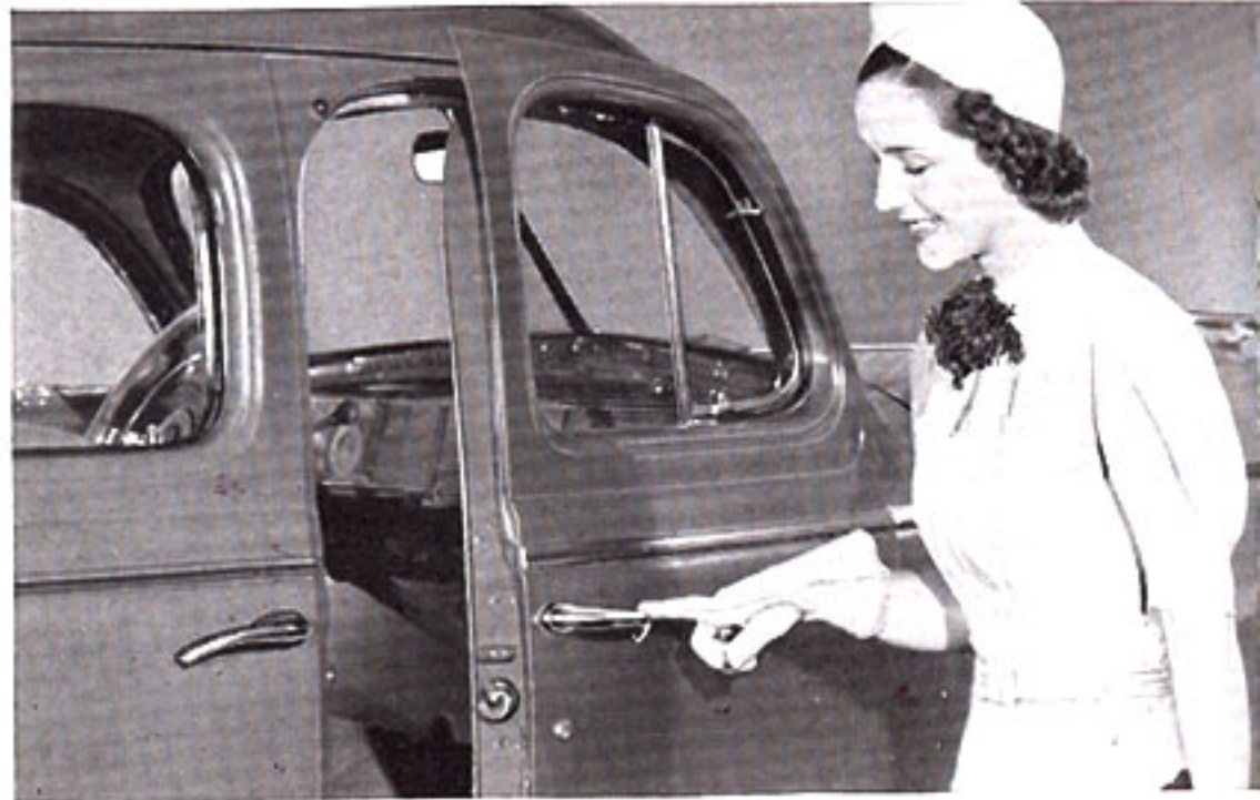
NON-SLAM DOORS equipped with new Rotary Door Locks may be closed with finger tip pressure. Door slamming is completely eliminated.
