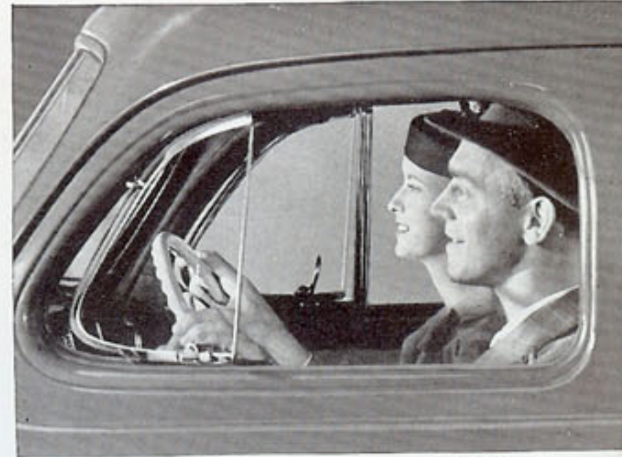
INDIVIDUAL VENTILATION is provided for front and back seat passengers. Air currents are controlled by these chrome-trimmed swing-type wings, front and rear.
