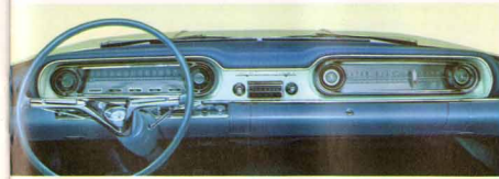
NEW TWIN-COVE INSTRUMENT PANEL has all the instruments—including a new resistor-type fuel gage and optional clock—looking you straight in the eye. Safety padding is standard on Super 88 and Ninety-Eight models.
