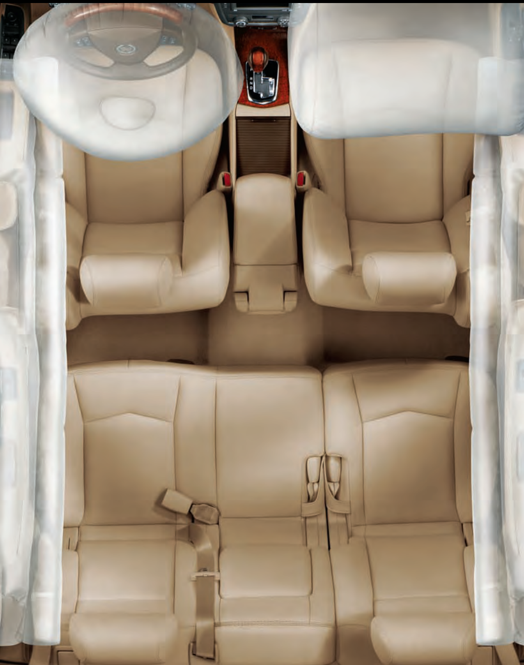
SRX features dual-stage frontal air bags, front seat-mounted side-impact air bags and front- and second-row head curtain air bags. †
