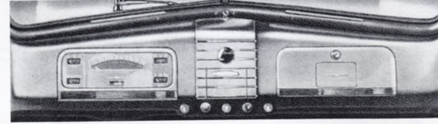
*INSTRUMENT PANEL —Clear-vision indicator dials are closely grouped in front of the driver. The ignition lock is illuminated. The Master De Luxe panel illustrated.
