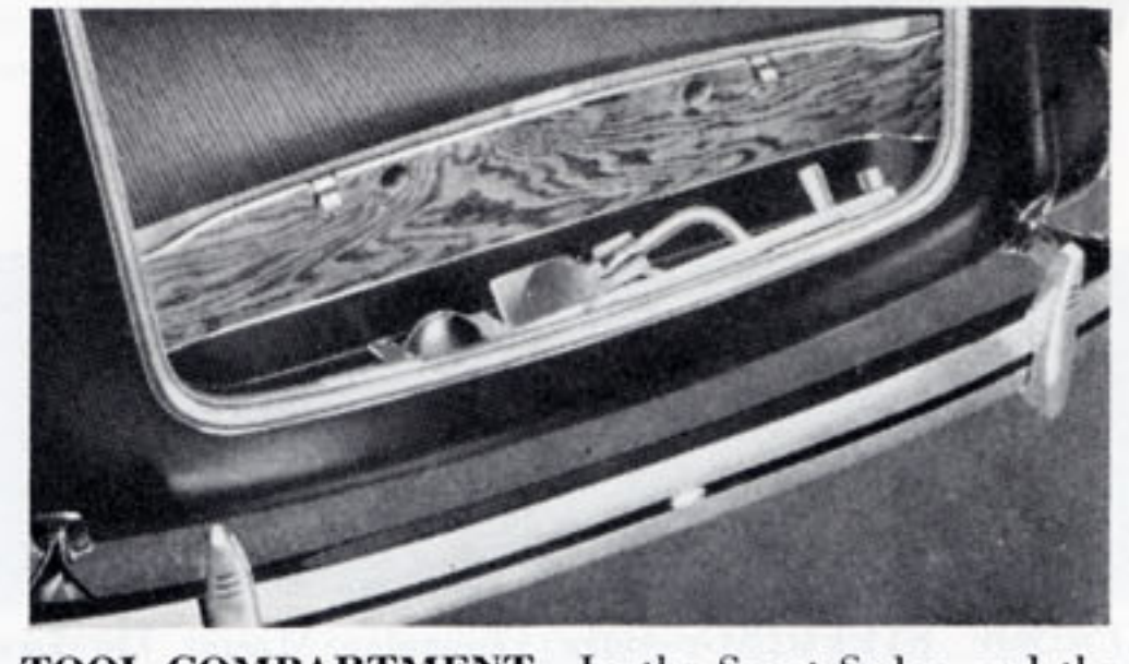
TOOL COMPARTMENT —In the Sport Sedan and the Town Sedan, tools are carried in an accessible compartment within the built-in trunk. Tools are protected by a floor-level cover, concealed by the floor mat.
