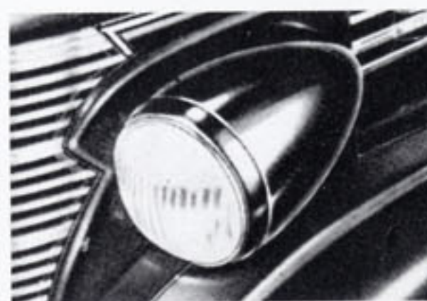
TEAR-DROP HEADLAMPS The slender lamps are mounted into the radiator shell in fixed position.
