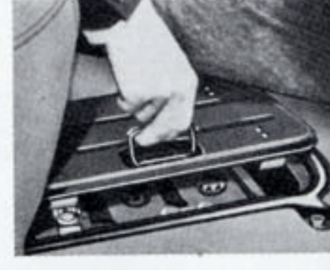
BATTERY —A snap-on rubber-sealed cover-plate makes the battery quickly accessible.
