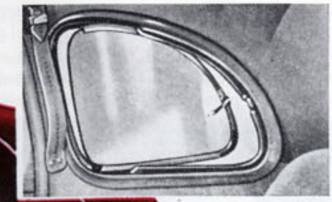
*TONNEAU WINDOWS Full-ventilating rear-quarter windows are found in the Master De Luxe Sedan and the Sport Sedan.
