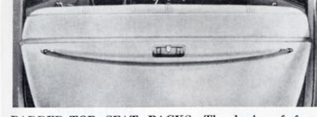
PADDED-TOP SEAT BACKS —The backs of front seats, in five-passenger bodies, are furnished with softly padded tops, as a measure of safety. All Master De Luxe five-passenger cars have robe cords.
