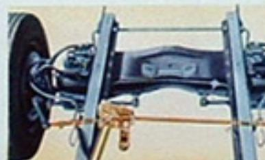
\*Knee-Action details (linkage, springs, built-in shock absorbers, ride stabilizer) are shown clearly above. In the view of the Knee-Action unit from above (left) is seen the improved shockproof steering, with a separate tie-rod to each wheel.
