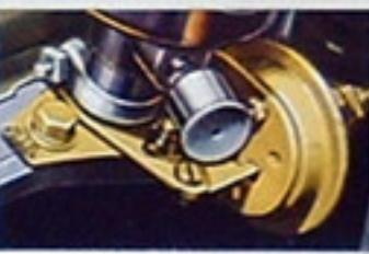
Air-pressure chambers in the fuel pump maintain a smooth flow of gasoline.
