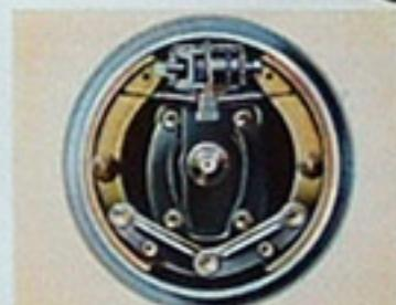
Double-articulated hydraulic brake-shoe linkage assures positive action and long wear by equalizing the pressure on the shoes.
