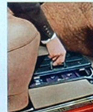
A snap-on rubber-sealed metal cover plate makes the battery quickly accessible.
