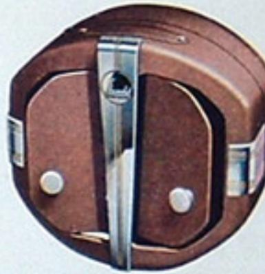
**BACK-UP LAMP**—For illuminating your driveway or other dark, confined areas, thereby reducing the hazards of colliding with unseen objects. Controlled by a convenient instrument panel switch.
