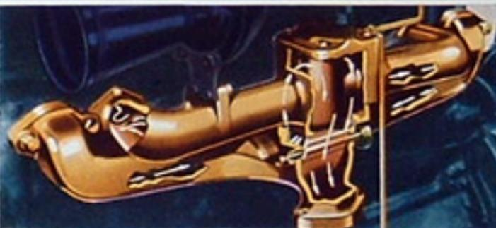
The temperature of the fuel mixture is regulated by a manifold warming chamber with automatic thermostatic control.
