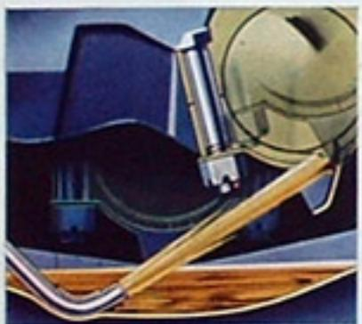
By pressure stream lubrication, an exclusive Chevrolet feature, connecting rod bearings are flushed with oil under high pressure.
