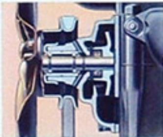
The leakproof ball-bearing water pump prevents loss of water and anti-freeze. It is self-adjusting and permanently lubricated.
