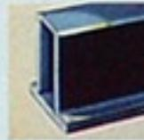
Box-girder construction, light and extra strong, is used in the chassis side-rails and cross-members. The side-rail bottom plate is welded to the stiffening flanges.
