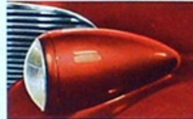
Slender headlamps are mounted on the fenders in fixed position.
