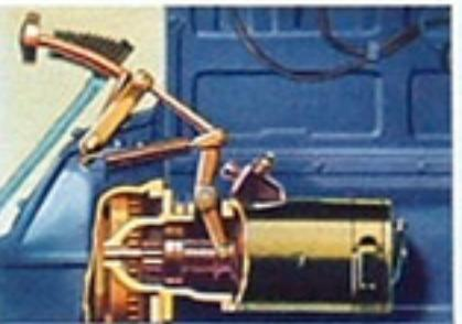
Mechanical starter engagement keeps the starter pinion in mesh with the flywheel until a positive start is effected.
