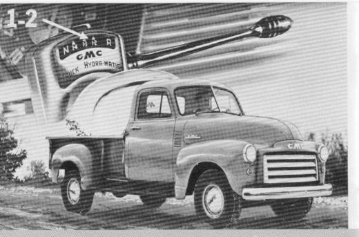
RANGE 1-2. Used when wheel slippage hinders starting, or where additional power, or braking, is needed. Truck starts in second . . . then, accelerator depressed for full power causes downshift to first gear.
