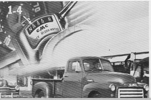
RANGE 1-4. For light traffic, suburban operation or open highway. Truck starts in first gear and shifts progressively through fourth, or high gear. You can rely on more positive drive . . . greater power when you need it!
