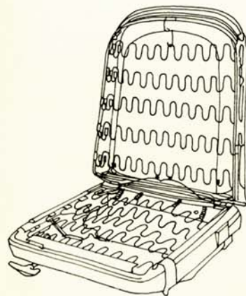
S-wire spring construction
