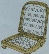
S-wire spring construction, foundation for Corvette's seating comfort
