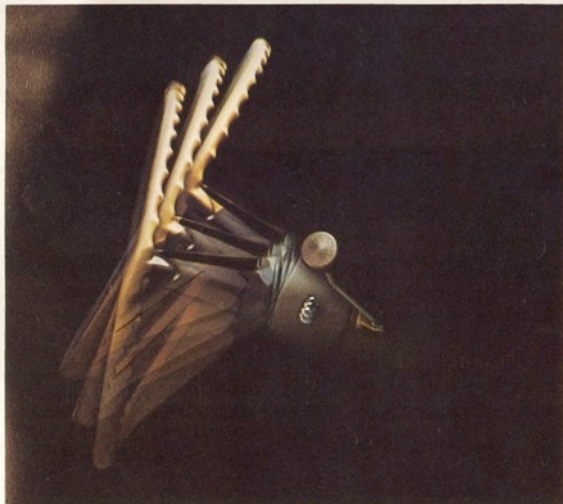
Specify the practical Comfortilt steering wheel; allows drivers sharing the same wagon to adjust wheel to any angle of seven they like best.
