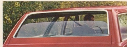
Power-operated tailgate window (standard on 3-seat models) activates from instrument panel and rear locations.
