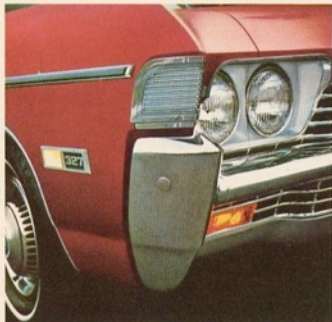
Standard side marker lights glow amber in front and red in back.
