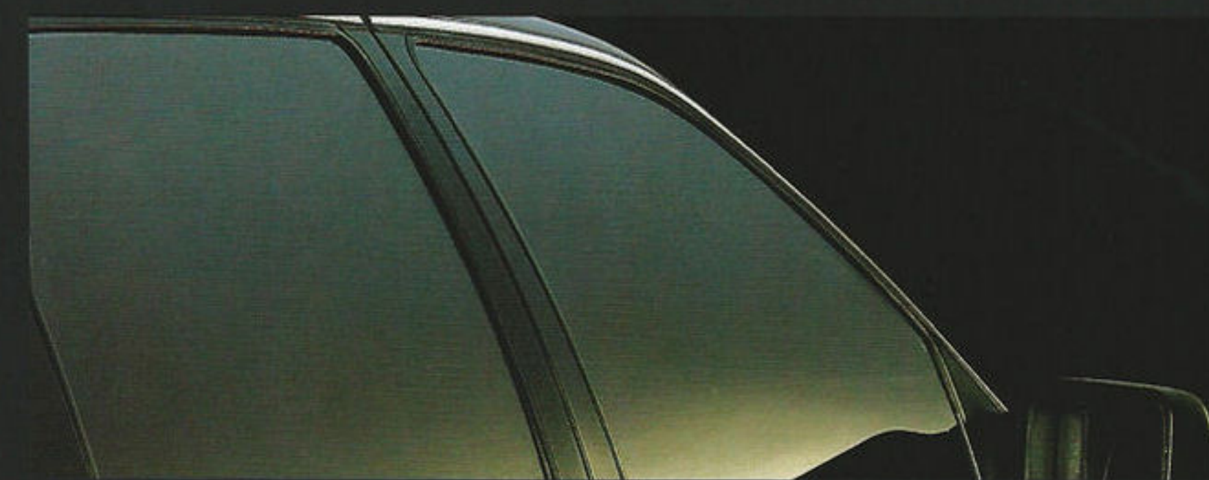
Flush mounted side glass improves aerodynamic efficiency.
