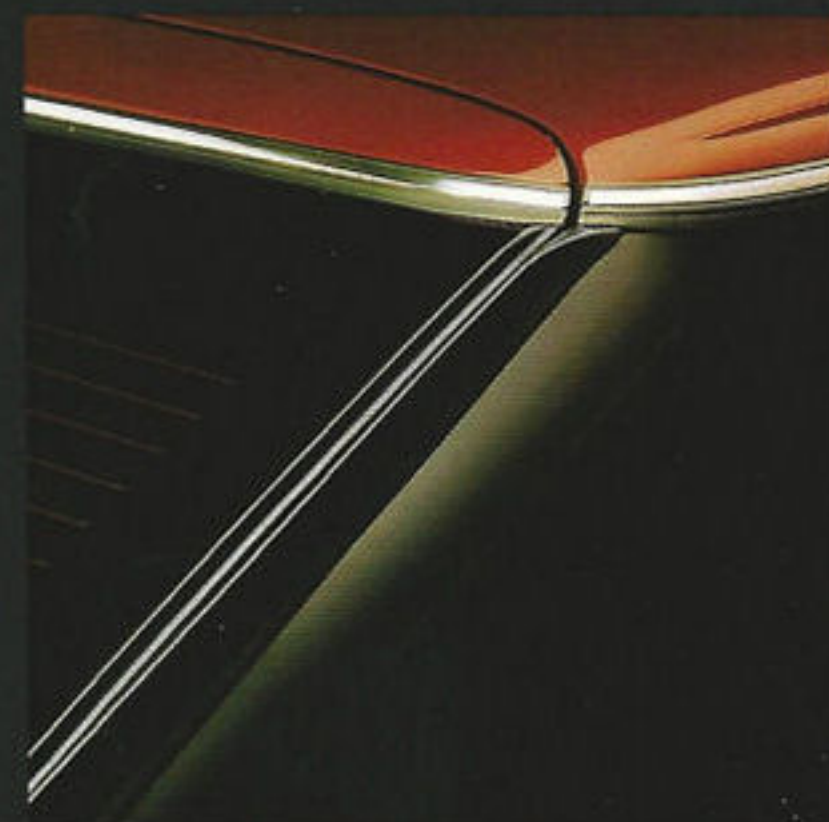
Strakes along the rear glass aid aerodynamics.
