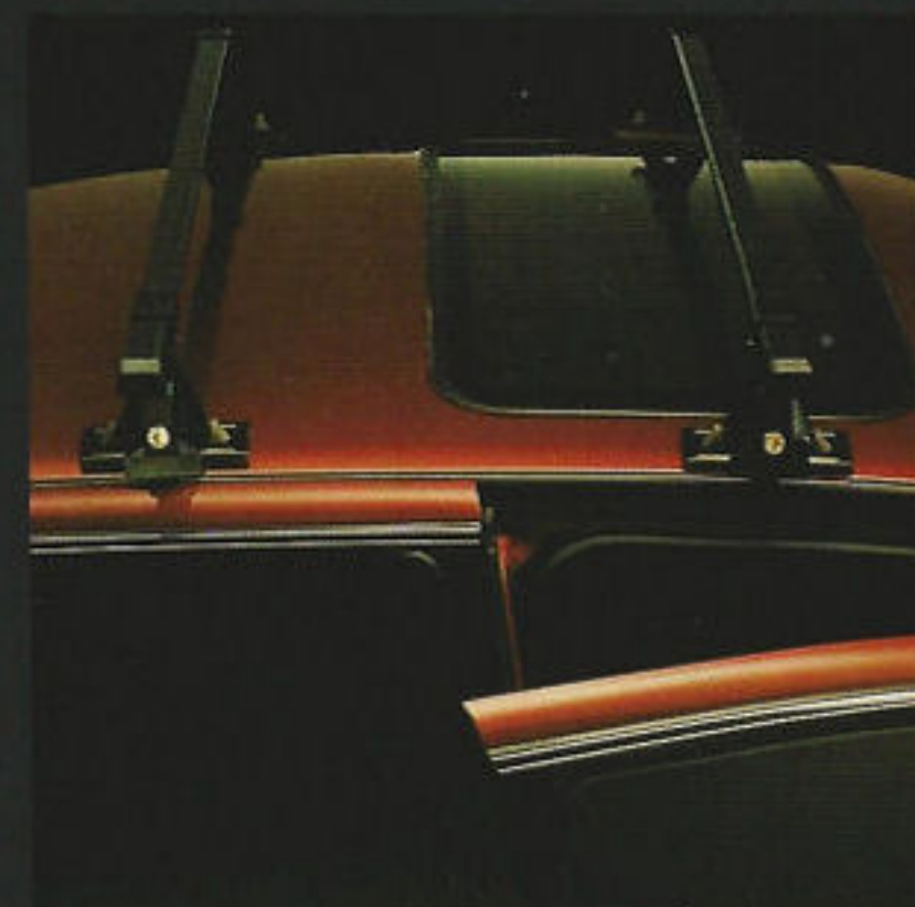
Special fittings allow the use of roof racks.
