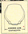
New wheel and rim construction increases volume of air in the tires without increasing size of tires. This means added stability and easy riding qualities. Five wire wheels are standard equipment at no extra cost on all Oakland cars.
