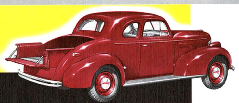
driver's compartment are similar to that of the *Master 85 Business Coupe* with pick-up box added . . . A rear deck lid is furnished for converting vehicle into a coupe . . . Wheelbase, 112 1/4 inches.
