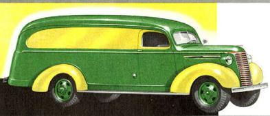
HEAVY DUTY PANEL—Capacity, 1½ tons . . . Large cargo space, with wide rear opening . . . Allsteel body, one-piece steel roof . . Full-length advertising panel . . . Wheelbase, 133 inches.
