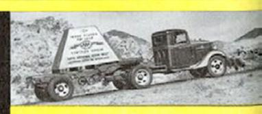
was demonstrated along a 3,511-mile route from Los Angeles to New York. Averaging 27.14 m.p.h., the *Heavy Duty* tractor unit, hauling a semi-trailer with a five-ton payload, established a record of 11.378 miles per gallon.
