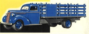
HEAVY-DUTY STAKE (158%' WHEELBASE)—Body specially adapted for heavy-duty work . . . Construction facilitates loading from sides as well as back . . . Stake sides supported in reinforced steel pockets guarded by a heavy rub-rail . . . Capacity, 1½ tons . . . Wheelbase, 158½ inches . . . Load space: 141½' long, 81½' wide, 38½' high
