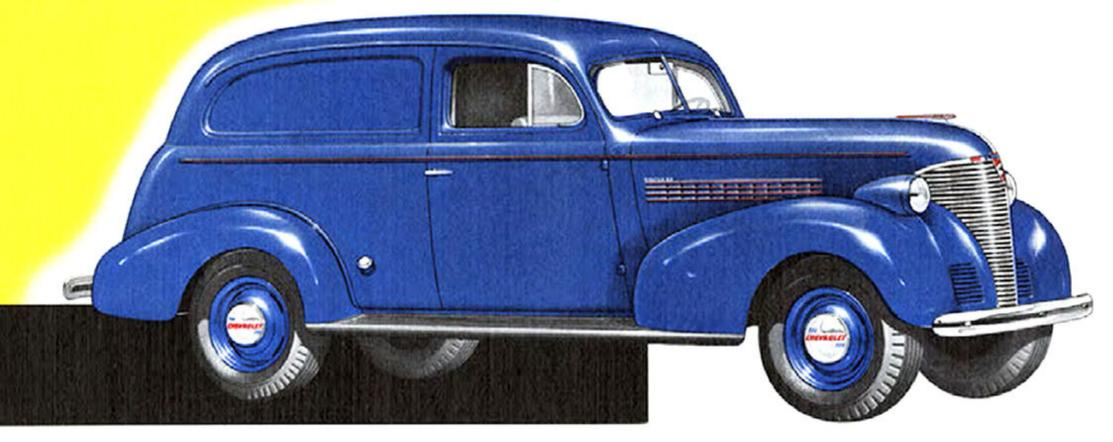
SEDAN DELIVERY—Special all-steel body mounted on the 1939 Master 85 passenger car chassis . . . Particularly recommended for easy riding, economy and speedy delivery . . . Hydraulic shock absorbers front and rear . . . Wheelbase, 1121/4 inches.
