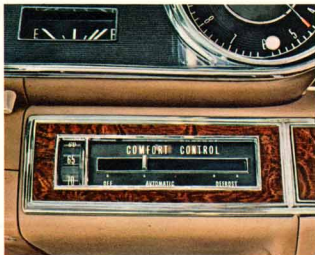
COMFORT CONTROL: Combines heating and air conditioning in a single unit. A dial permits setting of interior temperature as easily as with a home thermostat. Once set, the temperature is automatically maintained regardless of changes in the weather or the season.
