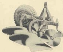
2-BOTTOM 12" GENERAL PURPOSE MOULDBOARD FLOW
