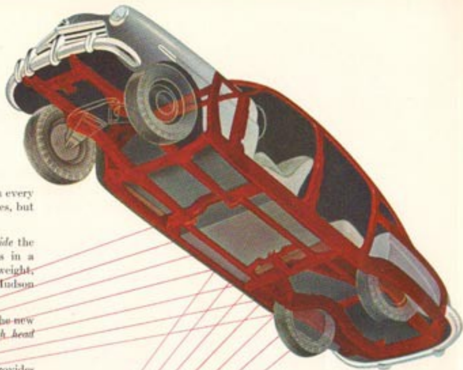
Underbody view, Hudson Monobilt body-and-frame. Box-steel foundation members, shown in red, provide girder protection all around, completely outside passenger compartments, and even outside rear wheels.
