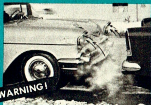
WARNING! Beware of carbon monoxide with front-end intakes.
