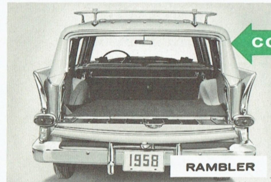
Rambler's tail-gate opening is nearly 4 feet wide with no hindering upper hinges or upper gate.
