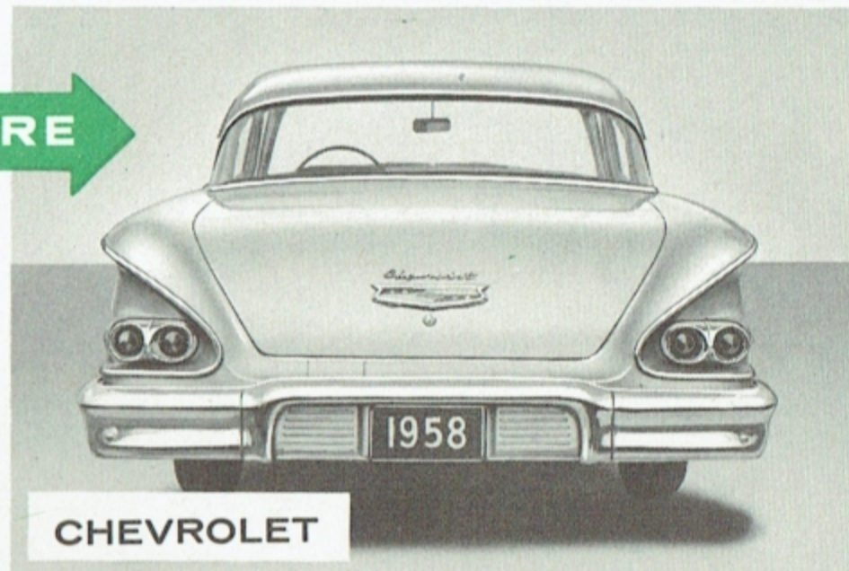
Lop-over fins increase width to 77.7 inches, about 4" wider than the '57 model, yet styling compromises force a trunk lid that makes loading difficult.
