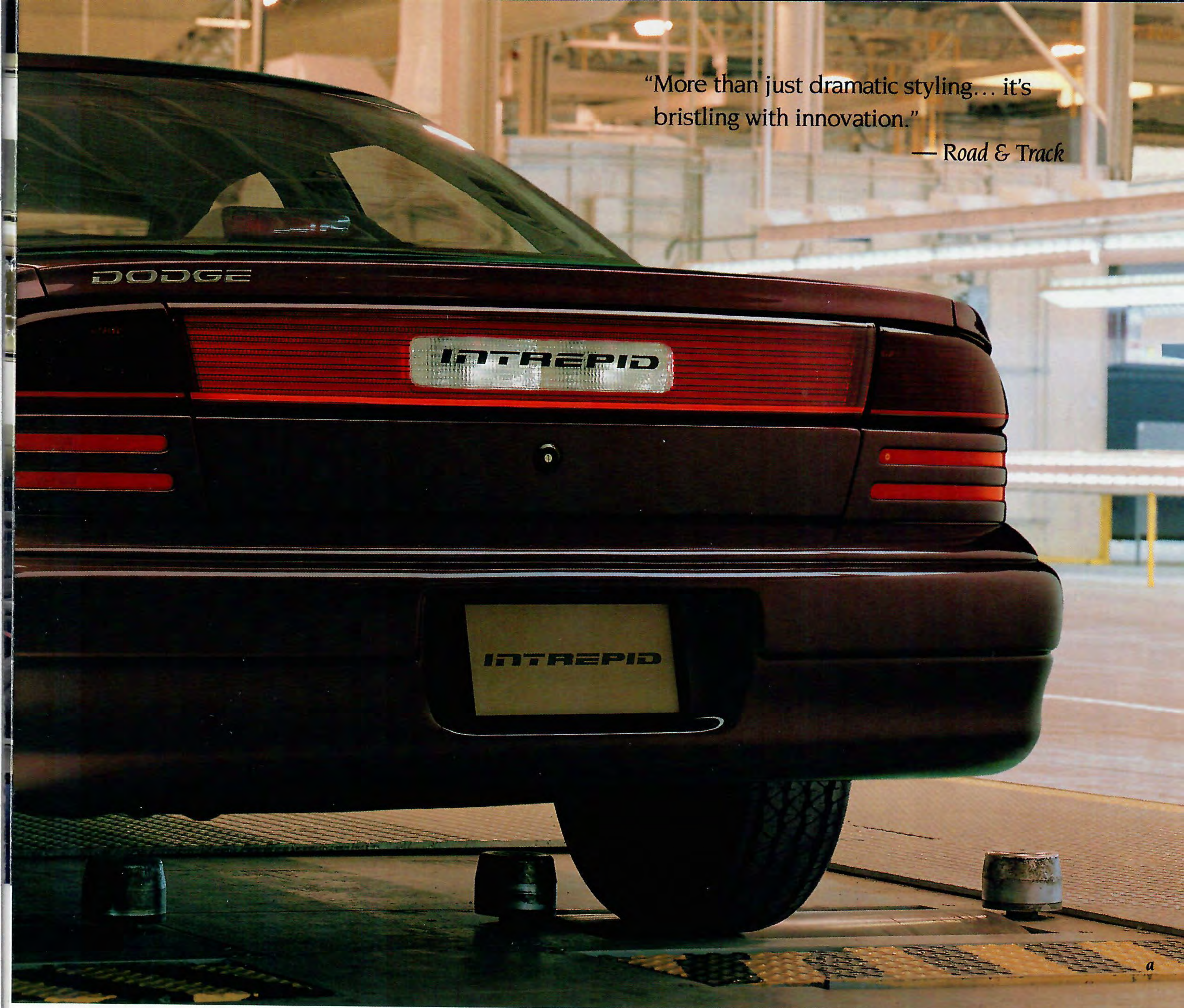
a) The power train and brake performance of every Intrepid is verified on a special computerized roller system before the vehicle leaves the Bramalea assembly facility.
