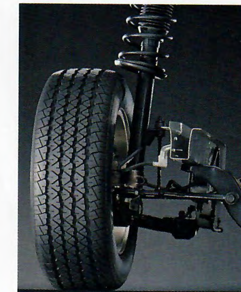
A four-wheel, fully independent suspension optimizes both ride and handling characteristics.
