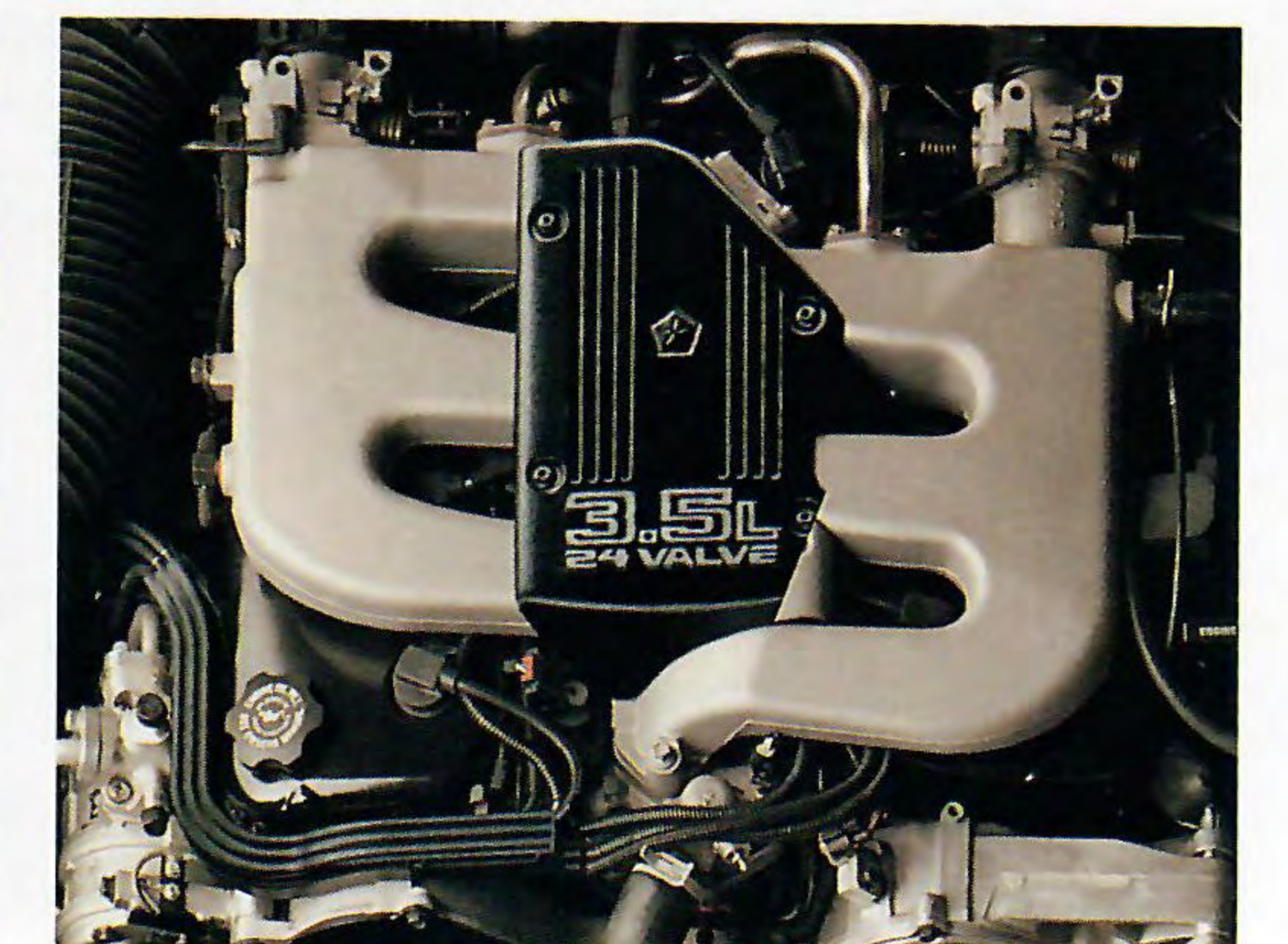
An available 214 horsepower, 3.5-liter V6 engine features an overhead cam design, 24 valves, sequential multipoint fuel injection and an active tuned intake manifold for smooth, responsive performance.
