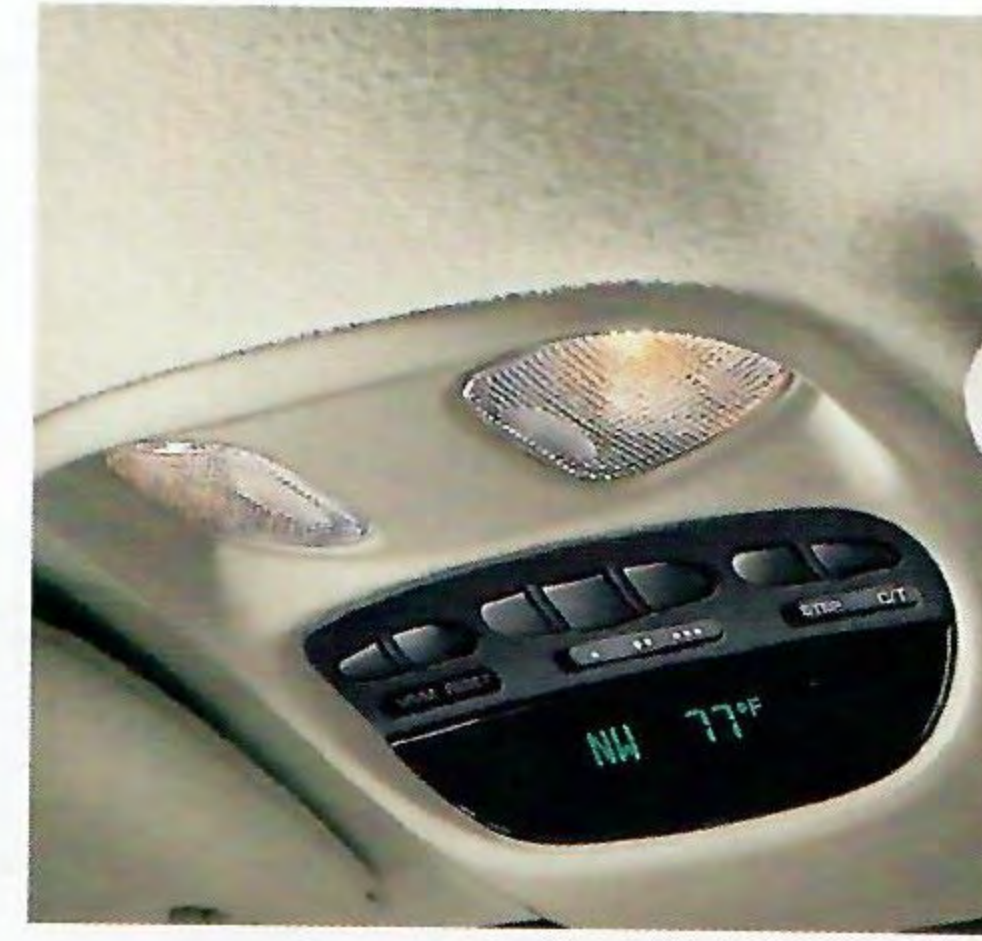
LXi's standard overhead console, with map lamps, compass, temperature, HomeLink® Universal Transceiver and trip computer functions, is also available on Concorde LXi.
