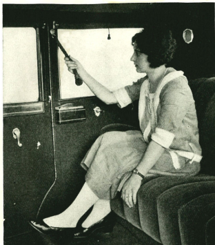
The cord to assist passengers in rising from the rear seats in Models 48, 50 and 51.
