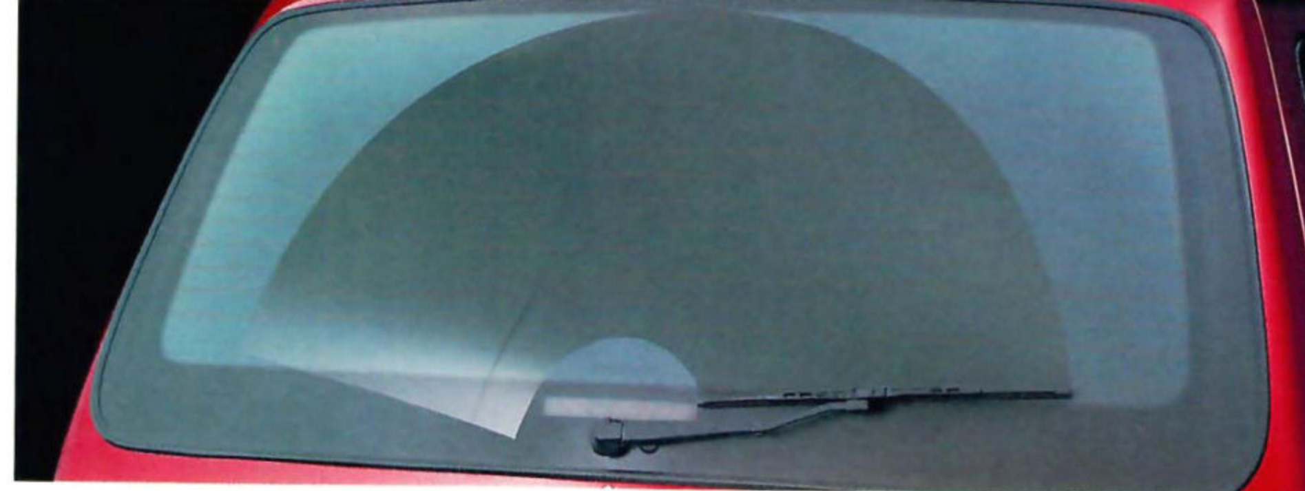
Standard liftgate fixed intermittent wiper/washer with dual nozzle wet arm washer clears Voyager's rear glass. The liftgate electric window defroster is standard on LE models, available on all other Voyagers.
