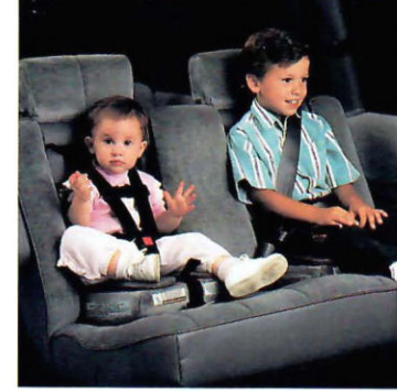
Both Integrated Child Seats offer five-point belt systems for use with toddlers, or the driver-side position converts to a booster seat for use with a standard Unibelt.
