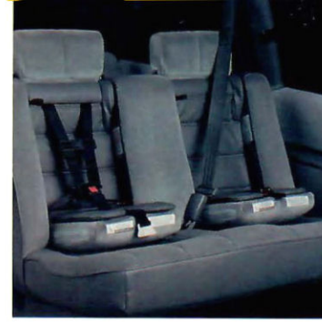
The Integrated Child Seats are available on all Voyagers with cloth interiors and meet or exceed FMVSS 213 Federal Safety Standard. Accommodates two adults when folded.
