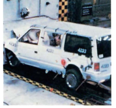
Crash tests evaluate bumpers, air bags, crumple zones and structural strength to create the safest minivans possible.
