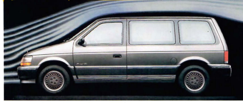
The new 1992 Voyager's rounded, contemporary styling and lower front end offer a sleek aerodynamic profile, while windshield pillar placement and generous glass area deliver excellent visibility.
