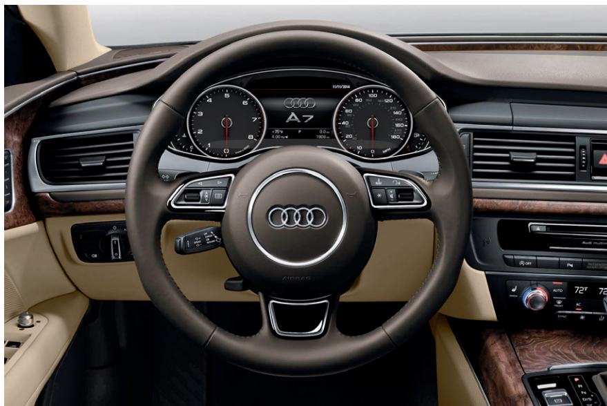
Three-spoke multifunction steering wheel with shift paddles and 7" color driver information system
