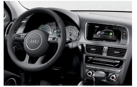
Q5 hybrid instrument panel with MMI® display showing hybrid drive modes
