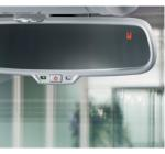
Auto-dimming interior rear view mirror with digital compass
