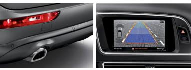
Parking system plus with front and rear acoustic Parking system plus with rear view camera parking sensors
