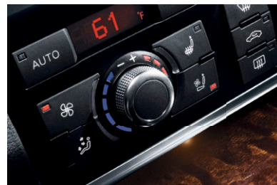
Front seat temperature controls
