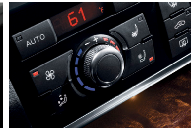
Front seat temperature controls
