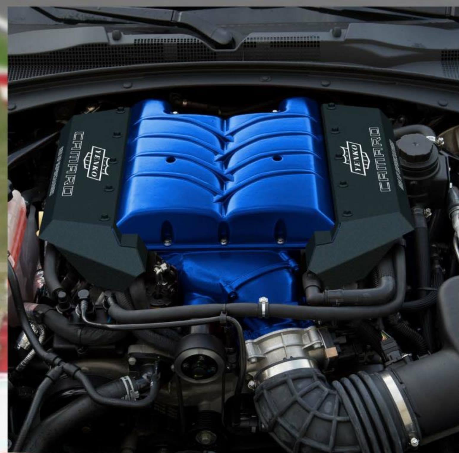
Specialty Vehicle Engineering's High-Output Supercharger shown with optional body color paint.
