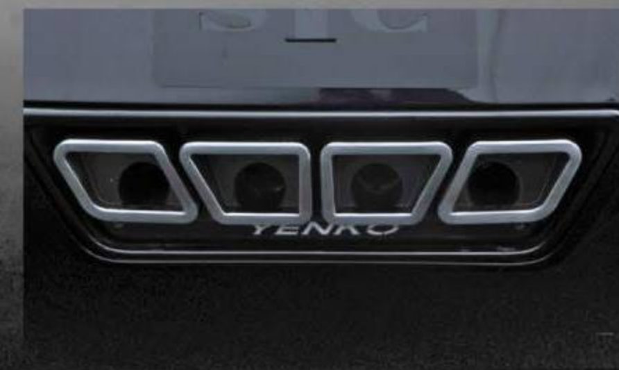
UNIQUELY-STYLED CAST ALUMINUM QUAD EXHAUST TIP WITH BRUSHED ALUMINUM FACE AND YENKO NAMEPLATE. (UTILIZES FACTORY DUAL-MODE EXHAUST)
