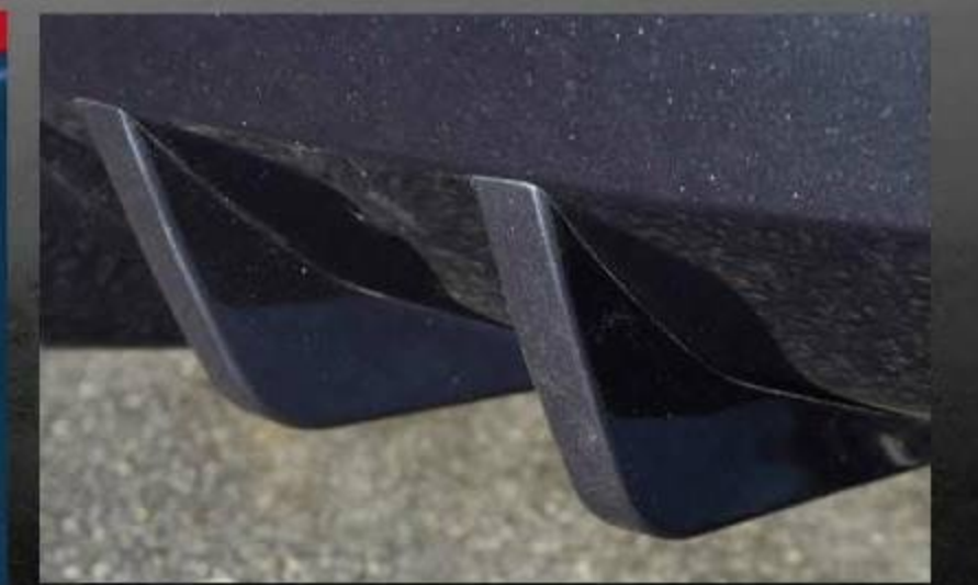
REAR DIFFUSER PAINTED IN CARBON FLASH METALLIC WITH FOUR DIFFUSER FINS
