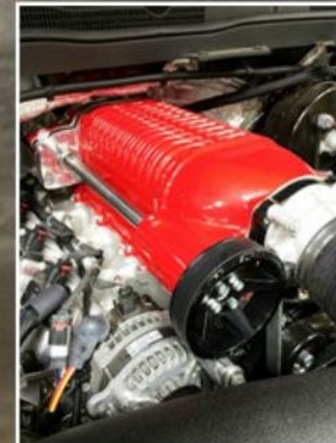
Specialty Vehicle Engineering's High/Output Series supercharged engine with 1000 horsepower and 875 lb.-ft. of torque. Shown with optional supercharger paint (black is standard).
