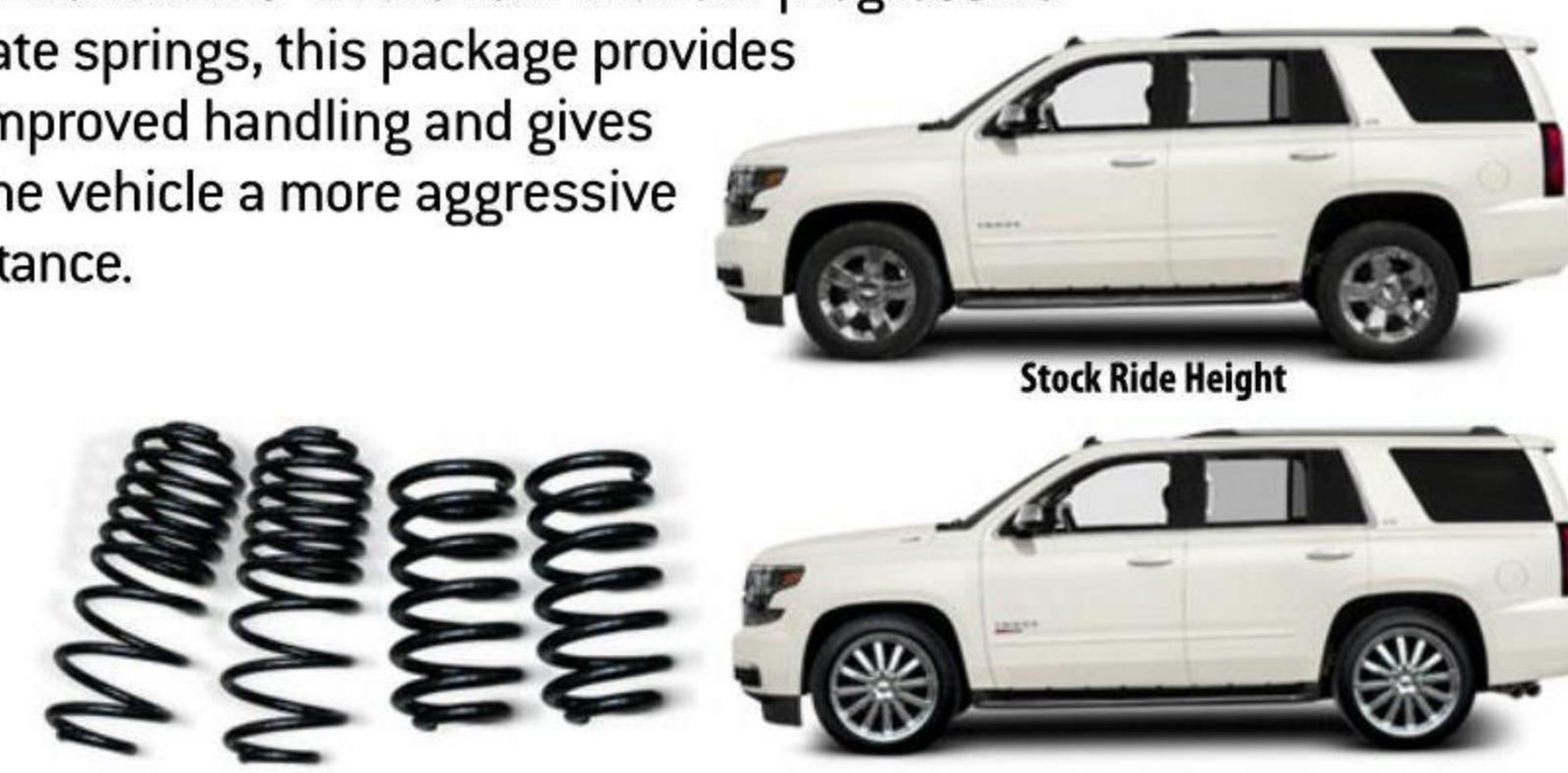
Lowered Ride Height with Specialty Vehicle Engineering Optional Sport Suspension Package
