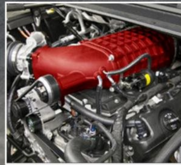
Specialty Vehicle Engineering's High/Output Series supercharged engine with 810 horsepower and 750 lb.-ft. of torque. Shown with optional supercharger paint (black is standard).
