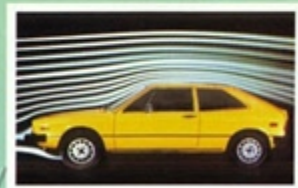
Aerodynamic Scirocco was designed in a wind tunnel.
