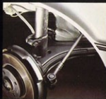
McPherson strut with long-travel coil/shock absorber.
