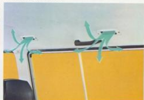
New ceiling vent louvers, right/left sides, are adjustable.
