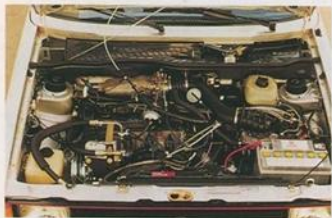
Transverse-mounted 1.8 litre engine features CIS fuel-injection, higher compression and a tuned exhaust system to deliver 90 horsepower. Shown with optional air conditioning.
