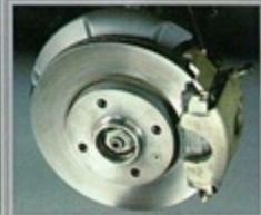
Disc brake with vented rotor.
