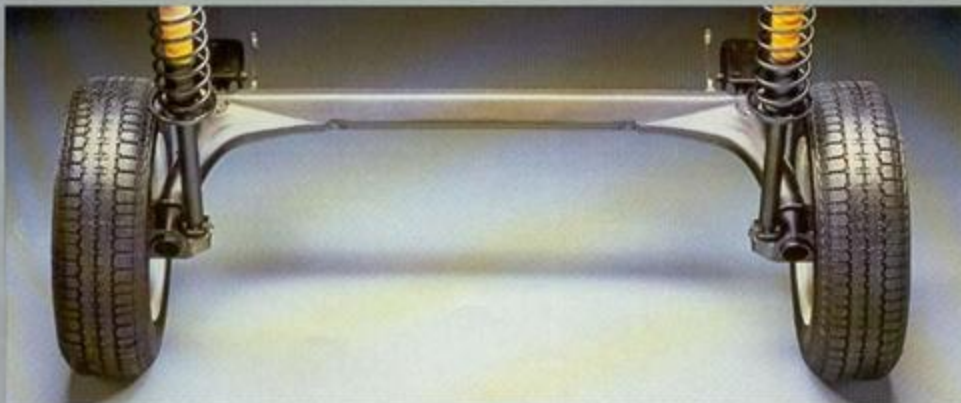
Linked trailing-arm rear suspension
