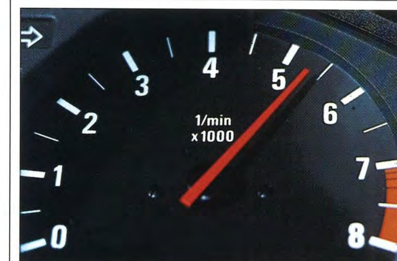
The red line on the tachometer starts at 7000 rpm. An engine speed governor cuts in smoothly and automatically as soon as this limit is exceeded. After all, you want to enjoy the M Power engine throughout a long and reliable running life.
