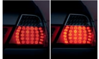
Adaptive Brake Lights increase the 3 Series Coupe's visibility by signaling the intensity of braking action.
