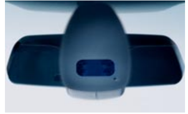
Rain sensor uses infrared light to measure the amount of rain. When the wipers are in the "intermittent" mode, the rain sensor automatically adjusts the windshield wiping interval as needed. Automatic headlight control (not shown), included with rain sensor, activates headlights by means of a sensor that responds to darkness.
