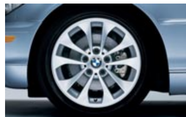
The 330Ci with 17 x 7.0 Double Spoke (Styling 98) alloy wheels and 205/50R-17 all-season tires. (Standard 330Ci; not available 325Ci)
