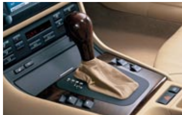
Five-speed STEPTRONIC automatic transmission provides a choice of three modes: "Drive," which incorporates BMW's Adaptive Transmission Control; "Sport" automatic, for a more dynamic shift pattern; and STEPTRONIC automatic, for the hands-on control of a manual without using a clutch (optional).
