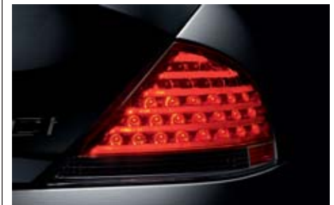
■ Adaptive Brake Lights help following drivers judge your braking situation. Under light braking, the lower three rows of long-life LEDs in the rear brake-light unit illuminate. During panic braking, Dynamic Brake Control (DBC) signals for the two upper rows of LEDs to illuminate.
