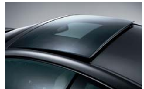
■ Tilting glass panel roof gives the interior an even brighter, more spacious feel. For greater ventilation, it tilts up; an electric sliding interior roof liner keeps the hot sun out. (645Ci Coupe only)
