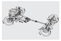
xDrive all-wheel drive system monitors readings from the DSC sensors and the gas pedal to determine if over- or understeer is occuring. This data is then used to continually vary power distribution between the front and rear axles, ensuring agile, neutral and forgiving handling at all times. (standard in 328xi; not available in 328i or 335i)
