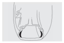
Run-flat tires allow speeds of up to 50 mph and travel up to 150 miles after a loss of air pressure. In situations that would normally result in a flat, reinforced sidewalls help prevent the tires from collapsing or loosening from the rim.
