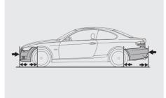
Impact-absorbing bumpers and compressible "crush tubes" front and rear help absorb the force of impact in collisions up to nine mph, helping to minimize damage to the vehicle's body and simplifying repairs. Only at higher impact speeds do structural supports begin to deform, dissipating impact energy to help protect occupants.
