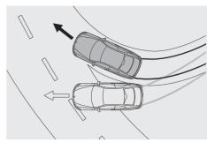
Dynamic Stability Control (DSC) with Dynamic Traction Control (DTC) features Brake Drying, Brake Stand-by, Brake Fade Compensation and Start-off Assistant. DSC is a braking control system that, when it senses an impending skid, helps to stabilize the 3 Series Coupe in just milliseconds. For sportier driving or in deep snow, the DTC system allows increased wheel slip.
