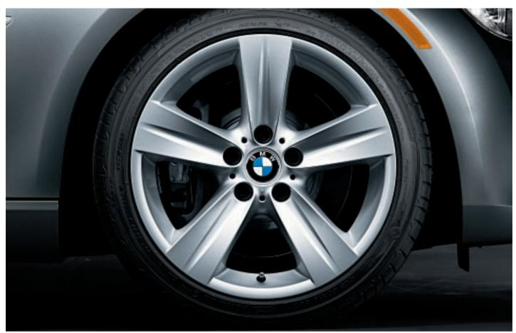
$\square$  Star Spoke (Style 189) light-alloy wheels and run-flat¹ performance tires.² In front:  $18 \times 8.0$  wheels and 225/40R-18 tires; in back:  $18 \times 8.5$  wheels and 255/35R-18 tires.³ (included in 335i Sport Package)
