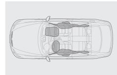
Six airbags, part of BMW's Advanced Crash Safety Management system, include "smart" dual-stage, dual-threshold front airbags that deploy at different forces, depending upon whether or not safety belts are worn; front-to-rear Head Protection System curtain-type airbags; and front-seat-mounted side-impact airbags.
