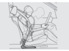
**BMW restraint system** for the driver and front passenger consists of a three-point safety belt, safety belt pretensioner and force limiter, all working in tandem for optimal protection in the event of an impact.
