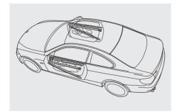
BMW's door-anchoring system includes a reinforcing bar with a hook-like member within each door. In a severe side impact, the reinforcing bar hooks the door to the body, locking them together to make a more rigid passenger cell. When the pressure is released, the anchoring system is designed to snap back so that the doors can open.
