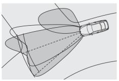
Xenon Adaptive Headlights illuminate the road ahead and to the side with brilliant clarity; Xenon headlights also have a dynamic autoleveling feature. BMW Adaptive Headlights illuminate the road around corners by directing the headlights into and through the bend, as soon as the vehicle begins cornering.
