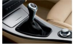
■ 6-speed manual transmission delivers a precise, athletic feel. Its responsiveness is due, in part, to the enhanced synchronization of shifts from neutral to each gear. A shortened shift lever and "throw" add to the sporty feel of the gearbox. The sixth gear drops revs at highway speeds for smooth cruising. (shown with iDrive, included with optional on-board navigation system)
