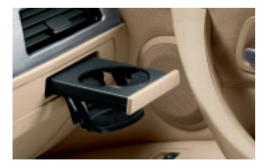
■ Cupholders are integrated into the dashboard, and can easily be retracted when not in use. (The driver's cupholder is not shown.) Two cupholders are also provided in the rear-seat center console, and one in the middle console for rear-seat passengers. (five cupholders, total)
