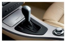
□ 6-speed STEPTRONIC automatic provides a choice of three modes: "Drive" with Adaptive Transmission Control; a more dynamic "Sport" mode; and STEPTRONIC automatic, for the hands-on control of a manual without a clutch. The 335i with Sport Package includes steering wheel paddle shifters. (shown with iDrive, included with optional on-board navigation system)
