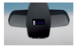
■ Rain sensor uses infrared light to measure the amount of rain. When the wipers are in the "intermittent" mode, the rain sensor automatically adjusts the windshield wiping interval as needed.
