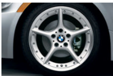
18 x 8.0 front/18 x 8.5 rear Bolted Star Spoke (Style 108) light alloy wheels and 225/40R-18 front, 255/35R-18 rear run-flat performance tires. 1 (Z4 Roadster 3.0si Sport Package)
