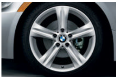
18 x 8.0 front/18 x 8.5 rear Star Spoke (Style 203) light alloy wheels and 225/40R-18 front, 255/35R-18 rear run-flat performance tires. 1 (Z4 Coupe 3.0si Sport Package)
