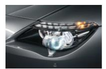
■ High-pressure headlight cleaning system helps keep headlights clear of ice, mud, road salt and other coatings, for maximum road illumination and enhanced driving safety.
