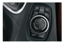
■ iDrive Controller, conveniently located on the center console, allows access to a variety of functions that are displayed on the Navigation screen. The turn/press button enables front-seat occupants to access the menu system and fine-tune settings for climate control, the audio system, and communication through BMW Assist.™
