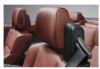
■ Integrated safety belt system provides optimal protection and ergonomic comfort for the driver and front-seat passenger. The seat-integrated design also helps make entering and exiting the rear cabin easier.
