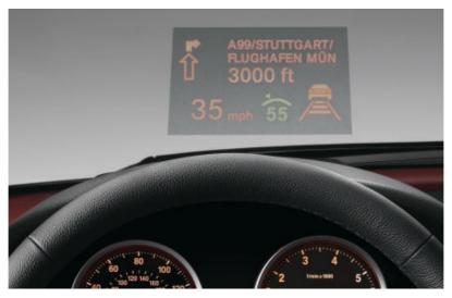
☐ Head-up Display projects important travel information, such as current speed, on the windshield directly in the driver's line of vision. Directional arrows from the Navigation system, Check Control data and optional Active Cruise Control³ functions can also be displayed. (note: Head-up Display not available with green band windshield)
