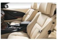
■ Eight-way power front seats with fourway power lumbar support and two-way adjustable headrests firmly support the driver and front passenger over long distances. Front-seat bolsters help eliminate "submarining" during sudden stops. Includes Active Head Restraints and driver's-seat memory function for settings. (shown in Cream Beige Pearl Leather upholstery)
