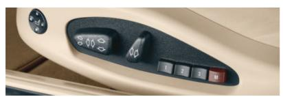
■ Power seat adjustments allow customized comfort for driver and front passenger. Three-setting memory system automatically adjusts the driver's seat, side-view mirrors and the steering wheel position.
