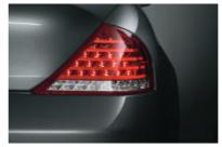
■ Adaptive Brake Lights help following drivers judge your braking intensity. Under light braking, the lower three rows of long-life LEDs in the rear brake-light unit illuminate. During panic braking, Dynamic Brake Control (DBC) signals for the two upper rows of LEDs to illuminate.
