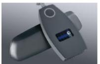
■ Rain sensor uses infrared light to measure the amount of rain. When the wipers are in the "intermittent" mode, the rain sensor automatically adjusts the windshield wiping interval as needed. Automatic headlight control, included with rain sensor, activates headlights by means of a sensor that responds to darkness.
