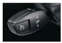
■ Cruise control lets you store and maintain a chosen speed above approximately 18.5 mph (activated via the left-hand side steering column switch). Cruise control is deactivated by applying the brakes or moving the lever.
