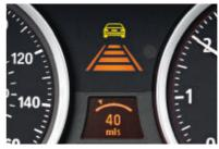
☐ Active Cruise Control (ACC) with Stop & Go¹ allows the driver to preset both a desired speed and distance. When ACC recognizes slower vehicles ahead, it reduces your speed to maintain the preset distance. Stop & Go can bring you to a complete stop if traffic calls for it. When you press the accelerator, ACC resumes your speed according to your presets.
