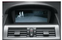
□ Night Vision is BMW's amazing system that helps you detect pedestrians or animals in the dark – up to 1640 feet ahead.<sup>4</sup> Using an infrared camera built into the front of the vehicle, you will be able to see potential road hazards displayed on your Navigation system monitor, and avoid them well before they are visible to the naked eye. At higher speeds, a digital zoom provides enlarged images of more distant objects on the screen.
