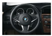
■ 3-spoke leather-wrapped multi-function sport steering wheel offers controls for audio system, cruise control and (accessory) phone. It also includes Voice Activation to let you keep both hands on the wheel while verbally adjusting various functions.
