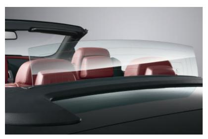
■ Heated glass rear window in the 6 Series Convertible can be raised independently of the softtop to reduce air turbulence and create a quieter cabin when driving at higher speeds. When driving in slower traffic, or when the softtop is raised, the window can also be lowered out of sight. (650i Convertible only)
