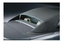
■ Automatic fin roof Convertible softtop is triple-lined and fully automatic. Simply press a button at the front of the center console to raise or lower. The top automatically unlatches from the header and folds down neatly. An interior lining helps reduce wind noise and enhances insulation. The heated glass rear window can be raised or lowered independently of the softtop. Available in Black or Gray. (650i Convertible only)
