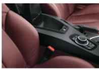
iPod and USB adaptor with cable connector lets you integrate the iPod, iPhone™ and other MP3 players into the audio system, and control various audio functions through the iDrive Controller or the multi-function buttons on the steering wheel.
