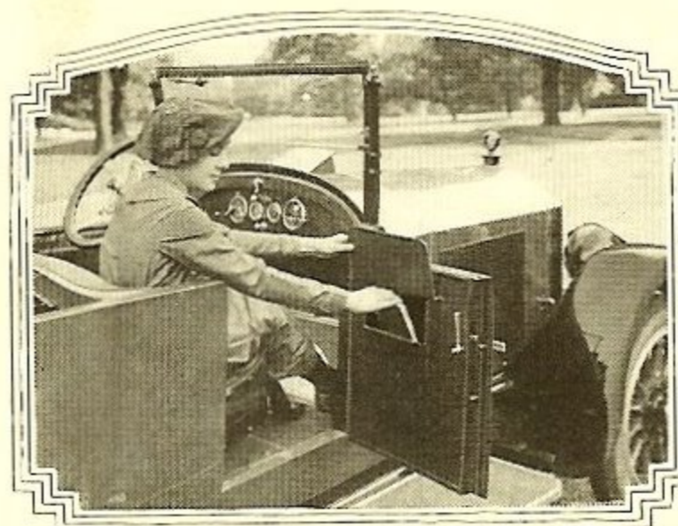
Spacious pockets are provided in the right fore door and both tonneau doors for the carrying of Blue Books, gloves, goggles and the other touring impedimenta
