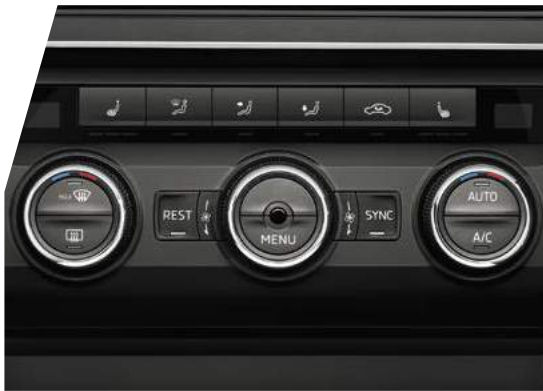
DUAL-ZONE CLIMATE CONTROL WITH HUMIDITY SENSOR
