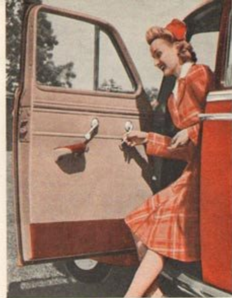
The characteristic good taste of all Studebaker design is apparent in the door trim of the 1942 Deluxstyle Champion. The fittings are of plastic and polished chromium. The padded arm rest serves as a door pull, and the leatherette toe panel protects the upholstery from being scuffed or marred by soiled shoes.
