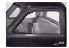
Perfect ventilation in any weather. Vertical metal division moulding lowers with window glass, affording free arm-room for signaling. Angle-set vanes may be kept open in driving rain - an exclusive feature. Comfortable in summer and winter alike.
