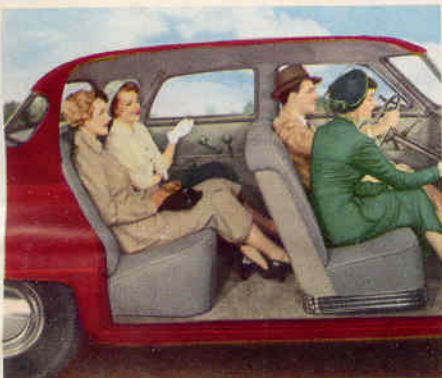
Rear seats are located well ahead of the rear axles where the ride is at its best.
