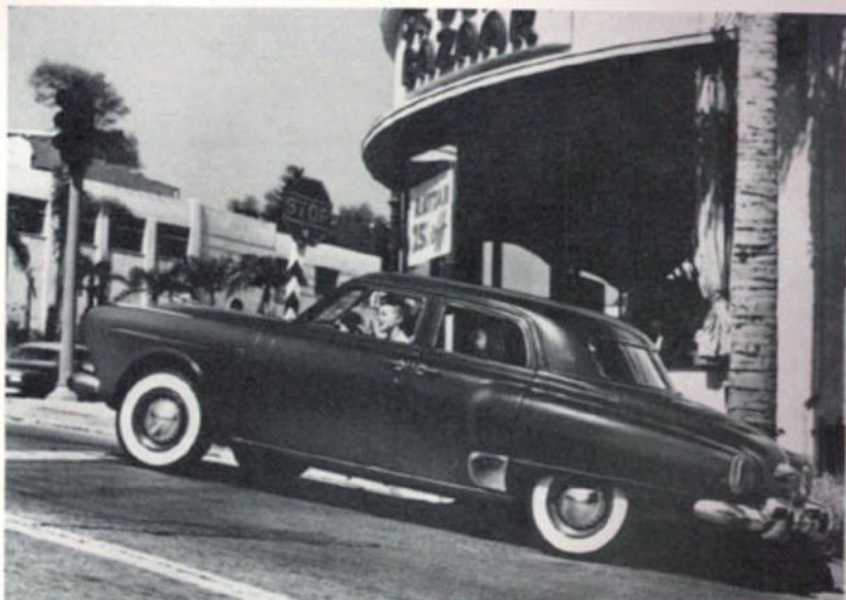
When the car is stopped going up hill Studebaker's hill-hobler keeps it from rolling back, while the driver takes his foot off the brake and uses the accelerator. While on an up-grade it holds in the hydraulic brake lines (as long as the clutch is thrown out) whatever pressure the driver has put on the brake pedal. Hill-hoblers are standard on Commanders and Land Cruisers; available at extra cost on Champions.
