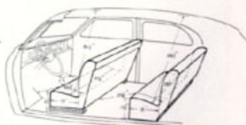
Four-door sedan. Doors, front 39½"; rear 30½". (Land Cruiser: Rear doors 34½"; legroom, front 40¼", rear 39¼"; seat depth, rear 19"; headroom, front 36½", rear 35". One-piece windshield.)
