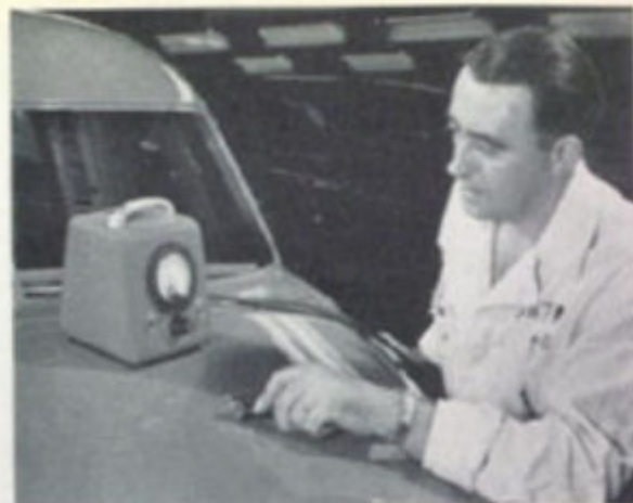
Cost of maintenance of the finishes for Studebaker bodies and sheet metal is kept at a minimum by extra-heavy coatings of color-fast, scratch resisting, hard-surface enamel—baked on, after all steel surfaces have been Blonderized as a rust preventive. Inspectors on the body assembly lines (above) check thickness of enamel with "paint meters."
