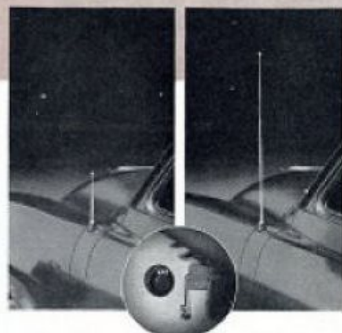
INTERNALLY CONTROLLED REEL-TYPE ANTENNA
