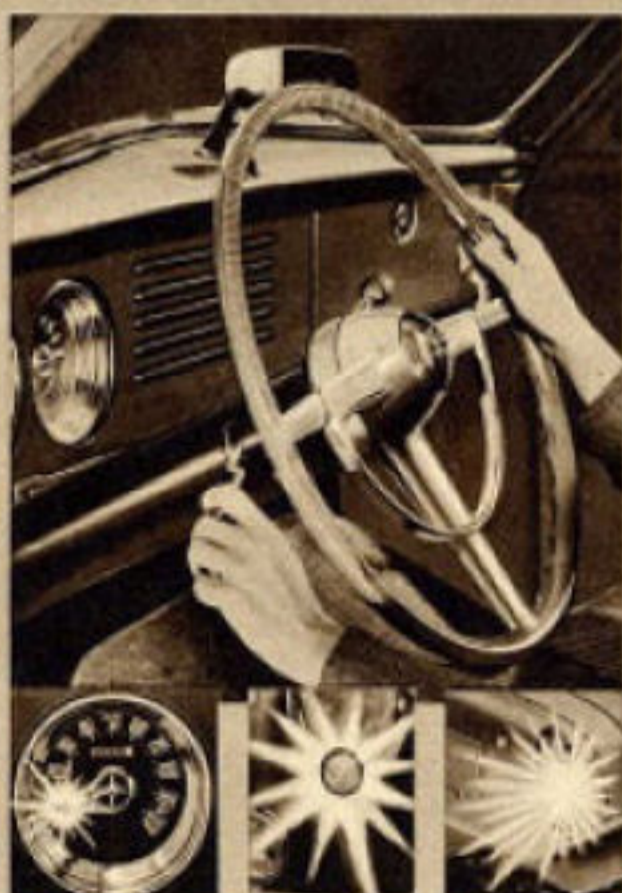
Directional signal equipment! Extra safety, comfort and convenience. For left turns, move lever backward and left front and rear lamps flash intermittently—for right turns, move lever forward.
