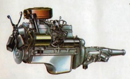
■ Super-economy on low-cost regular gas is provided by the sturdy Studebaker "6" engine. This gem of a power plant utilizes four massive main bearings for long life, new induction system and carburetion for amazing economy. It goes a long distance between fuel stops.
