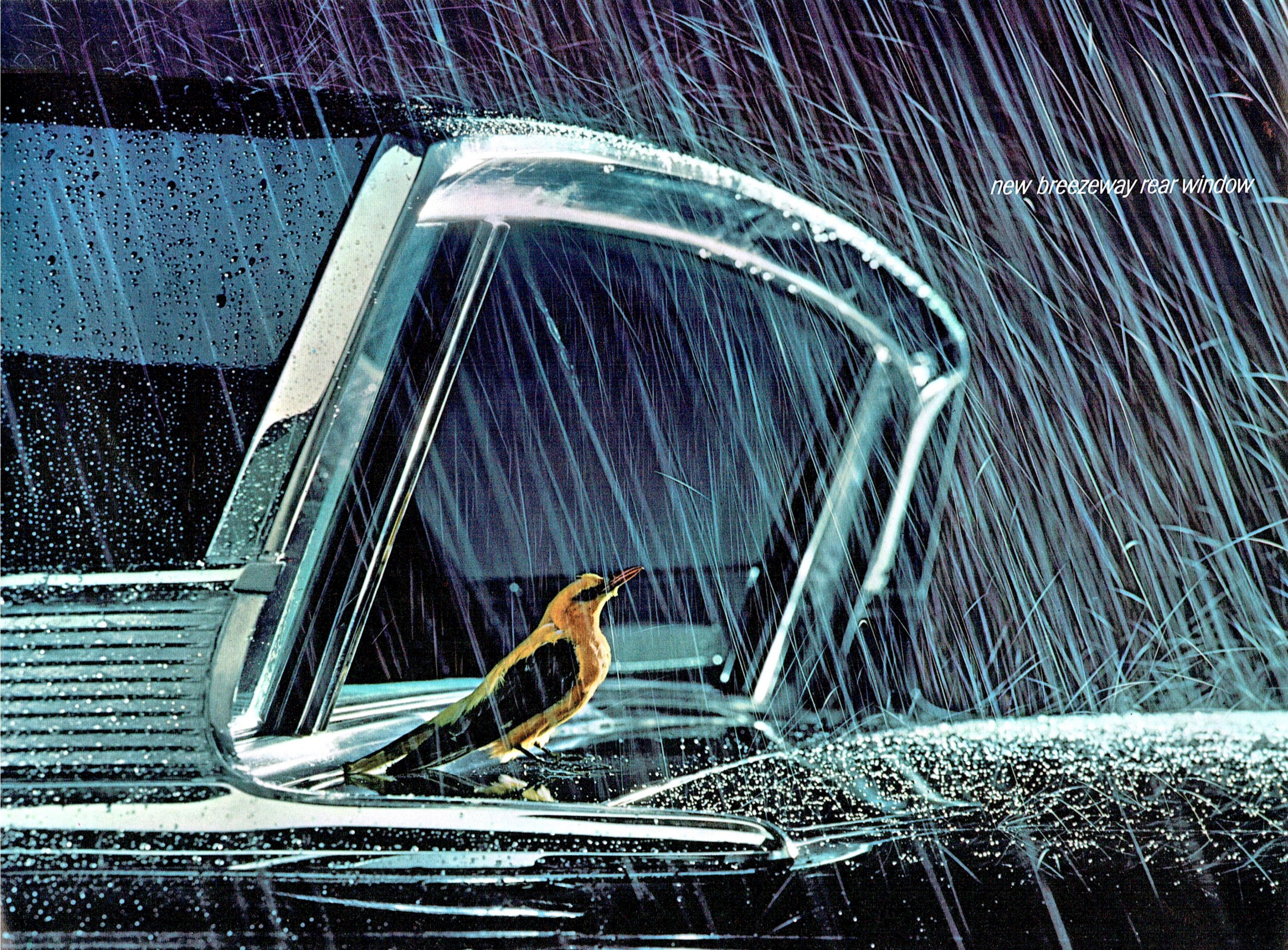
New Breezeway ventilation. Operates from driver's seat—window may be opened for maximum ventilation and comfort. Power control is standard in all sedan and hardtop models.
