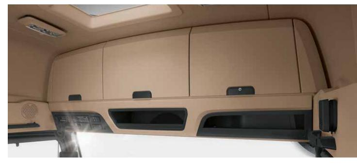
Stowage compartments above the windscreen. As a result of the new, symmetrical arrangement of the stowage compartments above the windscreen, the GigaSpace offers not only 332 I of stowage capacity, but also excellent freedom of movement and headroom on the co-driver's side. The upper stowage compartments with hinged lids are illuminated on the inside, lined with slip-resistant felt and offer two drivers adequate space for everything they need to take along with them.
