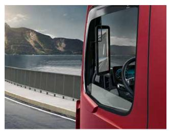
Side window wind deflector. The aerodynamically optimised tinted or clear side window deflector set for the driver's or co-driver's side protects against the airflow when driving with the windows open.
