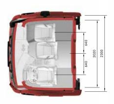
Engine tunnel: 170 mm Headroom over engine tunnel: 1460 mm
