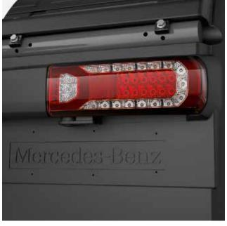
LED tail lamps. The new optionally available LED tail lamps set clear signals, especially the turn signal function, which features an outward-flowing light signal to indicate the direction.
