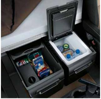
Drawers under the bed. The GigaSpace and BigSpace are equipped with two spacious drawers, one of which can optionally take the form of a refrigerator with a capacity of 36 I in which drinks bottles can be carried standing upright<sup>2)</sup>.
