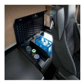
Exterior stowage compartments. With a capacity of up to 420 I, the two stowage compartments located under the bed in the L-cabs can be accessed from both the inside and outside and offer a huge amount of stowage space. Two adjustable stowage trays are optionally available to allow better use to be made of the space.
