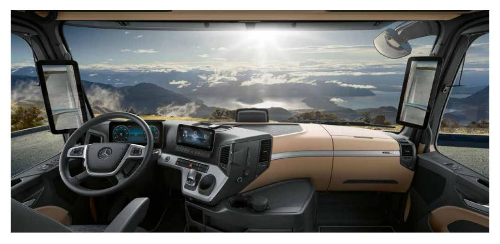
Multimedia Cockpit<sup>1)</sup>. The new Actros features the innovative Multimedia Cockpit for enhanced driving comfort, ergonomics and ease of operation. The new, state-of-the-art workplace comprises four screens in all. The primary colour display and the secondary Multi-Touch-Display, each with a screen diagonal of 10", can be operated via the new multifunction steering wheel with Touch Control Buttons.
